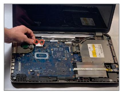
Disconnect the two antenna cables connected to the WLAN card.
