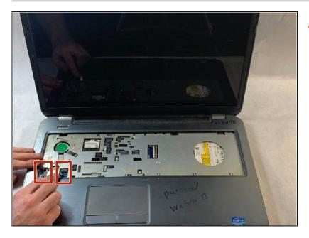
Using your fingers, unplug the two palmrest ribbon cables found at the bottom left of the integrated keyboard's slot.
