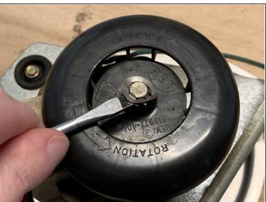
Use a flathead screwdriver or a small pry tool to carefully pry off the circular clip from the cooling fan.
