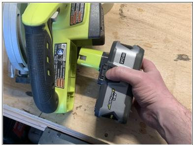
Unplug your circular saw or remove the battery before replacing the blade!
