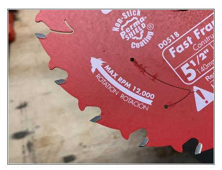
When inserting the new blade, be sure to note its rotation and install it in the correct orientation.
