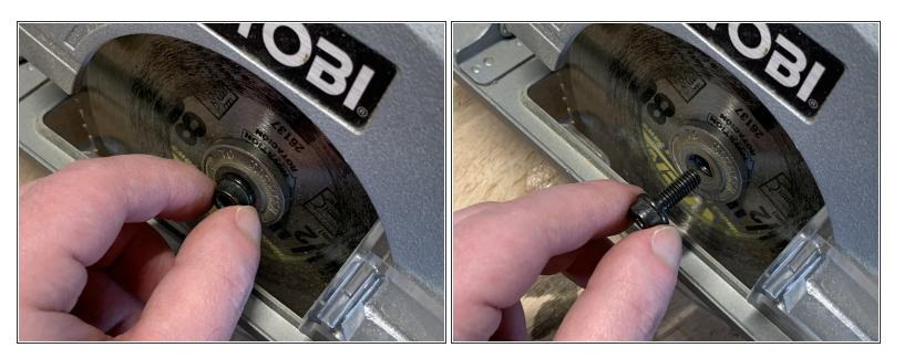
Once loosened, continue unscrewing the bolt with your fingers and remove it from the saw.
