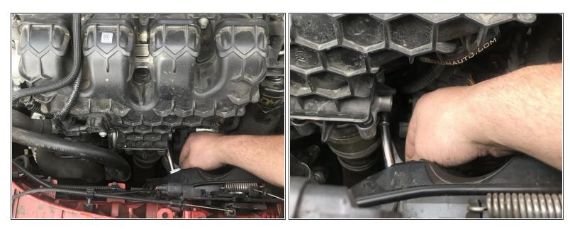
Using a 1/4 inch 7mm deep socket and 1/4 inch flex head wrench, loosen the worm clamp on the cold air intercooler pipe.
