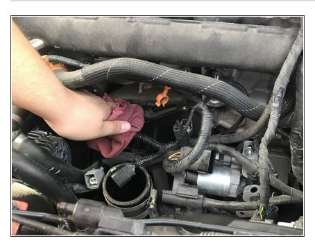
Wipe down the mounting surface and the inside of the PCV plate with a shop rag.
