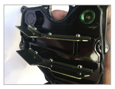
Remove the PCV plate and the old PCV plate gasket.
