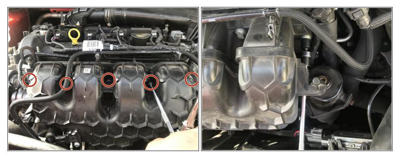
Using a 1/4 inch 10mm wobbly socket, 1/4 inch 8 inch extension, and 1/4 inch ratchet, remove all 5 of the cap screws holding the intake to the cylinder head.
