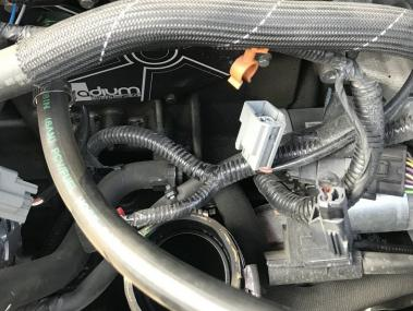
Unplug both left and right engine ground strap connections.
