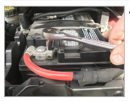
Using a 1/4 inch flex head ratchet and a 1/4 inch shallow 10mm socket, loosen the battery cable tightening nut.
