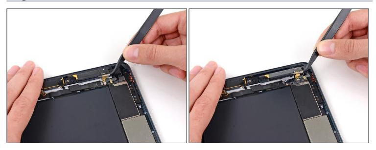
• Use <u>tweezers</u> to lift and remove the top right antenna from the rear case.
