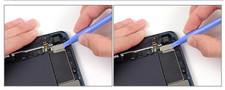
• Use a plastic opening tool to push the metal bracket slightly to the left.
