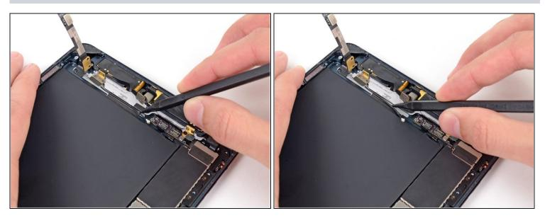
Use the tip of a spudger to peel back the tape securing the top left antenna cable to the rear case.
