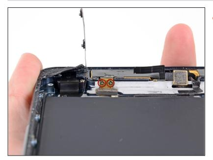
Remove two 1.5 mm #00 Phillips screws securing the side of the top left antenna to the rear case.
