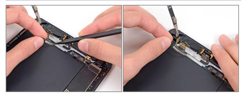
While gently pulling up on the top left antenna cable, continue using the tip of the spudger to separate the tape from the rear case.
