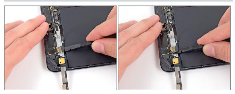
Slide the flat end of a spudger beneath the top left antenna's screw tab, separating the small bit of adhesive holding it in place.
