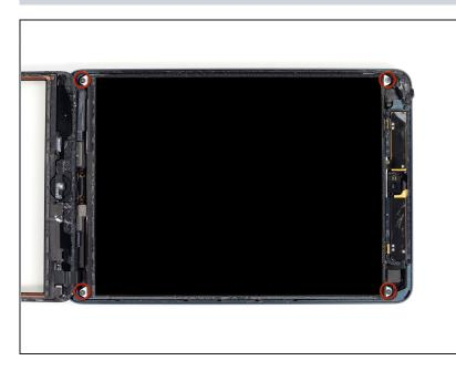
Remove the four 3.9 mm Phillips #000 screws securing the LCD to the rear case.
