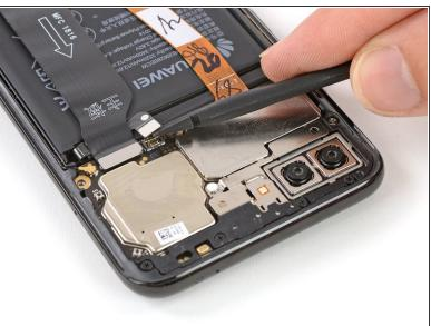
Use a spudger to pry up and disconnect the battery flex cable.
