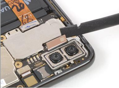
• Use the flat end of a spudger to pry up and disconnect the flex cable for the rear cameras.
