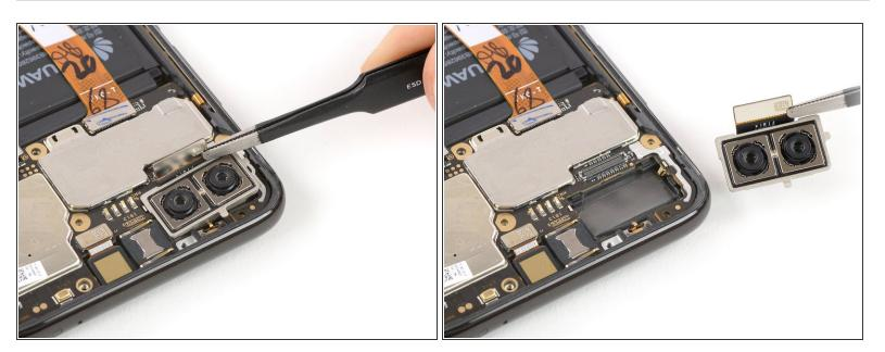
Use a pair of tweezers to remove the rear cameras.
