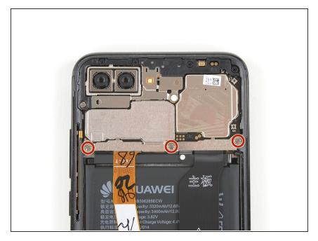
Remove the three Phillips #00 screws (2.9 mm length) that secure the metal bracket on top of the battery, interconnect, and display flex cable.
