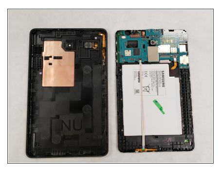
• Remove the LCD assembly from the housing and place it face down on the table.
