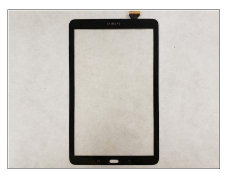
Once the ribbon cable is removed, pull the screen off of the motherboard and place it to the side.
