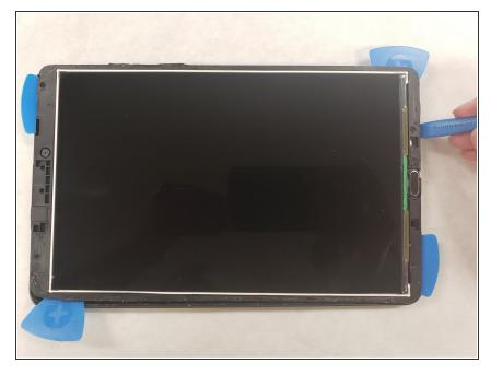
• Continue along the outer edge of the housing until you have placed an iFixit opening pick in each corner.
