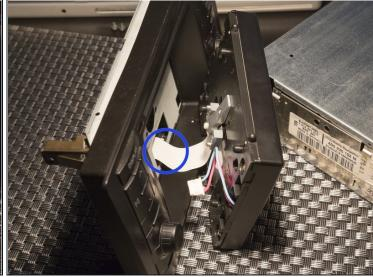
• Remove two 4 mm T10 Torx screws.
