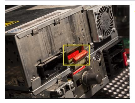
Use a spudger to disconnect the cable connecting the GPS with the radio unit.
