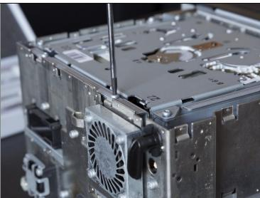
• Remove five 6 mm T9 Torx screws from the top side of the unit.
