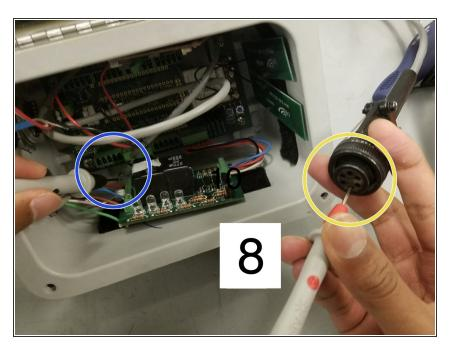
8. Confirm there are no breaks in the wiring between the interface board the autosampler. See this <u>tutorial</u> for more details.
