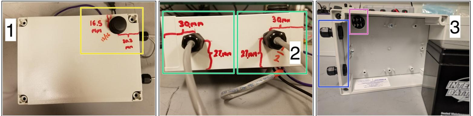
1. Drill a hole in the top right corner 16.5 mm from the top and 30.3 mm from the side using a 13/16 inch drill bit.
