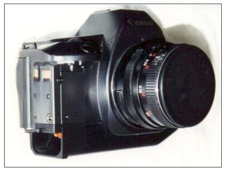
• With the 2-Cent coin you can open the battery case and remove the battery. The screws in this section will be removed with the smaller one (#00) of the two crosshead screwdrivers.
