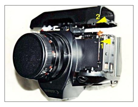
This picture shows the result of performing the next step, and why special care is needed. The bottom plastic cover is held in place by a small plastic loop (2) that engages a lug (1) on the front cover. All these parts are plastic and can be easily damaged.
