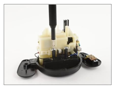
The motor assembly is attached to the base with three screws—two in the front and one in the back.
