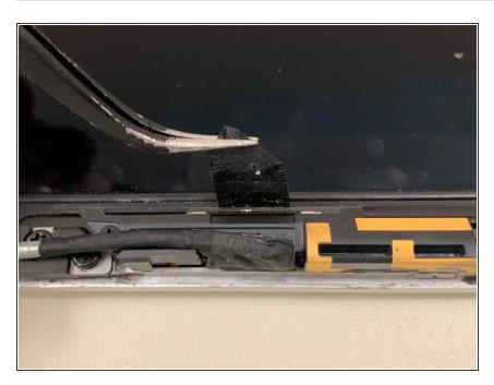
Peel up the tape covering the cable connector.
