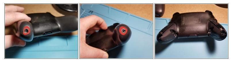
The left and right grip screws are held in place with one J00 screw each. After the screw is removed, the grip slides straight off.
