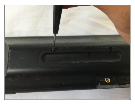
Use a phillips tip screwdriver to open the battery panel.
