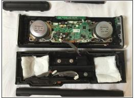
• Use your fingers to remove the back enclosure. Unplug the cabels before removing it completely.
