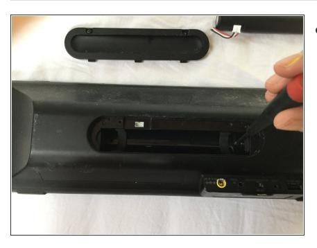
Under the battery there are two phillips tip screws. Remove them to continue to the motherboard disassembly.
