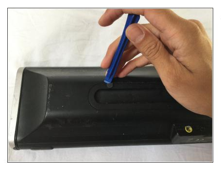
Start opening the battery panel by removing the two rubber seals.
