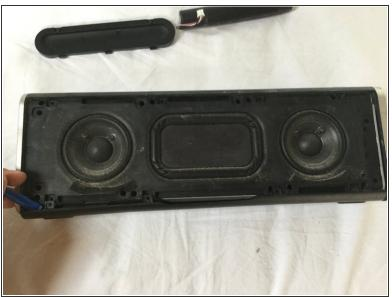
Gently pull down the bottom enclosure and remove it.
