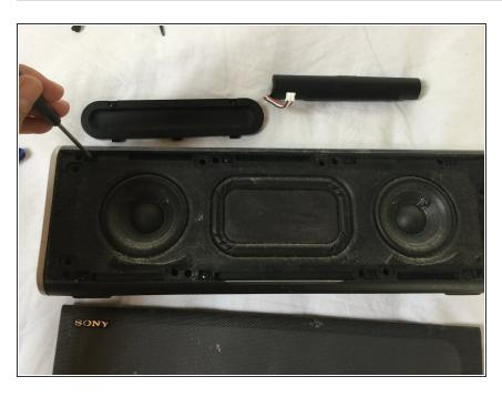
Use a phillips screw driver to remove all the visibel screws. There should be 17 screws.
