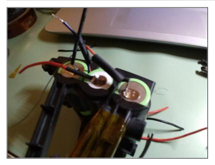
Slip the heat shrink, as best you can, over both joints and shrink 039
