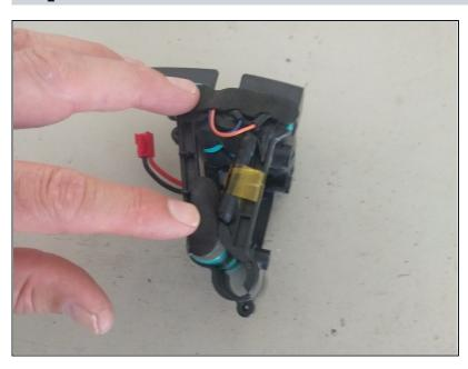
Note locations of insulating tape and remove them, two from each side. 016 HEED WARNING ABOUT SHOCK!
