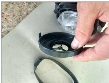
• Remove gasket and fan shield 010-011
