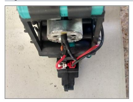
Disconnect red battery connector and white motor connector 009
