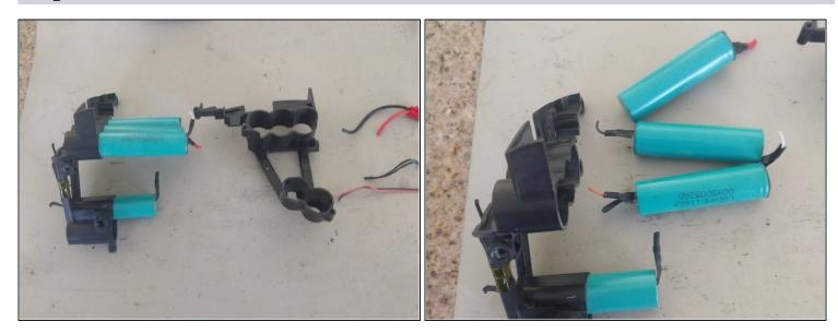
• Slide the right side plastic carrier off of the batteries. 023 Note that two connectors are loose. So that you can determine the orientation of the batteries (where + or - goes) in the carrier, maintain the orientation while you slide the three batteries out of the left carrier. 024
