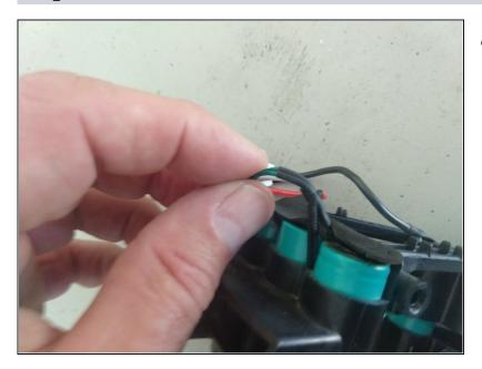
Pull temperature probe, that is connected to two green wires, out of assembly 017
