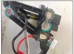
• Cut thin ORANGE wire about a cm from heat shrink. cut thin BLUE wire about a cm from heat shrink. 018 cut thin WHITE wire about a cm from heat shrink. cut thick BLACK wire about ½ cm from heat shrink. 019 cut thick RED wire about ½ cm from heat shrink. 020
