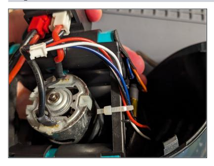
Lift motor assembly from plastic body. Clip tie-wrap 008 and disconnect small white connector from electronics board 007 (picture 008 disappeared, but the tie wrap is the only one in there)
