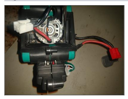
• Remove two (2) screws to remove motor 012
