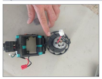
Note the holes into which motor mount screws go 013
