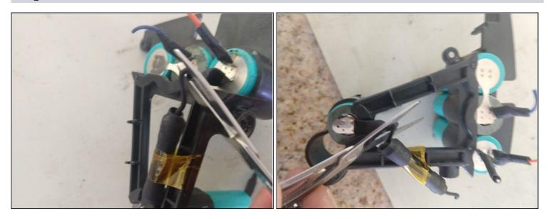
• cut thin BLACK wire from fuse next to the battery heat shrink (two places) 021-022
