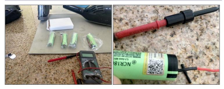
• Take the old batteries to the place where you recycle batteries. Unpack and check voltage of new batteries (NCR 18650B, 3.6V, 3000mAhr, welded on leads, voltage less than 3V probably indicates a bad battery) 025-026
