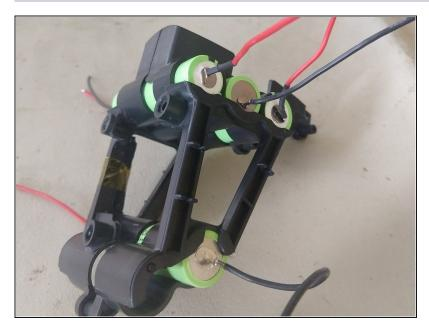
Put the right half of the carrier over the batteries and slide into place. Do not put in the screws, yet, you still need to put in the button and the electronics. 028
