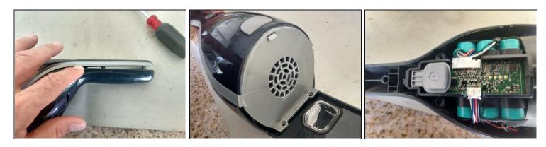
• Split case 005 and lift off 006 revealing electronics board 007
