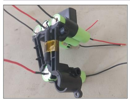
Put the new batteries into the left half of the carrier, ensuring the + of the battery is in the same direction as its predecessor. 027
