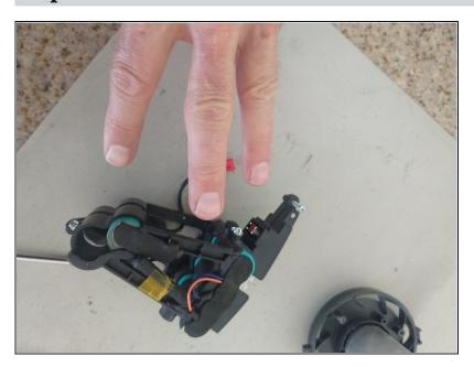
Remove three (3) screws from the battery carrier 014
