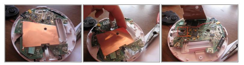
• Now for the other side. Carefully peel up the antenna plate so you can get at the other data ribbon.
