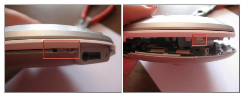
• Insert the tip of a screwdriver between the white upper layer and the gray lower layer. Carefully pry apart. There are small clips that help hold the two layers together and you don't want to snap them.
