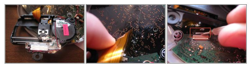
Now to remove the laser reading assembly. Carefully peel the orange data ribbon off the circuit board to the plug. Using the flat screwdriver, pry the black clip away from the tan part.
