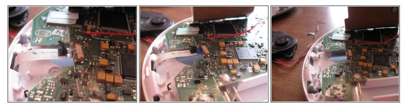
Peel the black tape off the plug. Pry up with a screwdriver on the brown clip and remove the data ribbon.
