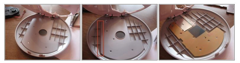
Now for the top layer. unscrew the five screws and place them on the magnet. Pry up on the side indicated to remove the cover.
