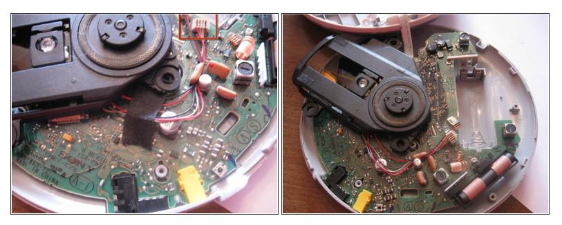
• Now for the power wires. Pry up on the side opposite of the wires.
