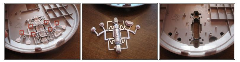
• To remove the buttons, carefully pry up around the little pins and pull up.
