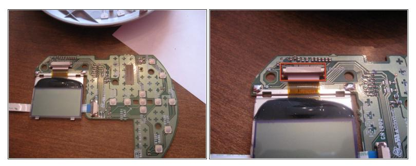
Pull out the circuit board and LCD screen assembly. Pry up on the brown clip to remove the LCD screen.
