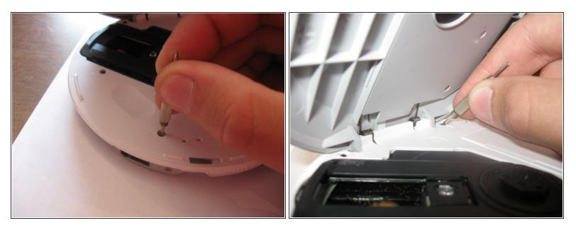
Unscrew the six screws and place them on the magnet so you'll be able to find them later. Sony was nice enough to put the screws next to the lid at an angle so you can fit a screwdriver in there.
