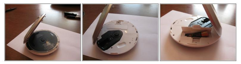
• Open it, remove any CDs and put away. Open the battery cover and remove the battery.
