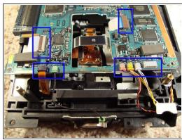
Before flipping the board and see where all the fun takes place we need to unplug a few connectors that transport data form the circuit board to the optical drive.
