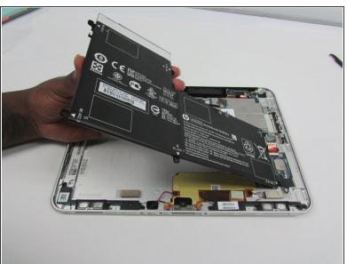
Carefully lift the battery away from the bottom cover.
