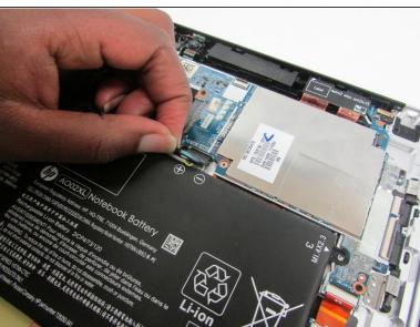
Disconnect the battery to system board connector by pushing gently on it with a plastic pry tool and then pull it away from the system board.
