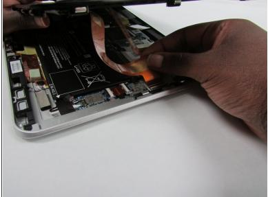
Release the ZIF connector to which the display cable is attached, and then disconnect the display cable from the system board.
