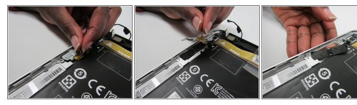
Remove the volume button board and cable.
