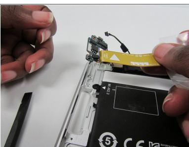
Remove the power button board and cable.
