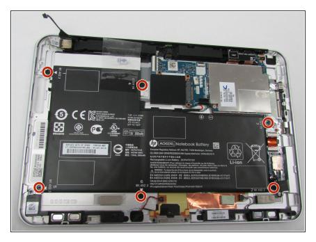
Using a philips 00 screw driver take out the six Phillips PM1.3×2.0mm screws
