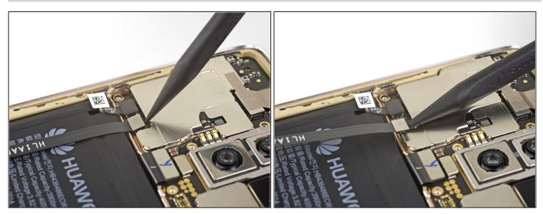
Use the point of a spudger to pry up and disconnect the fingerprint extension cable from its motherboard socket.
