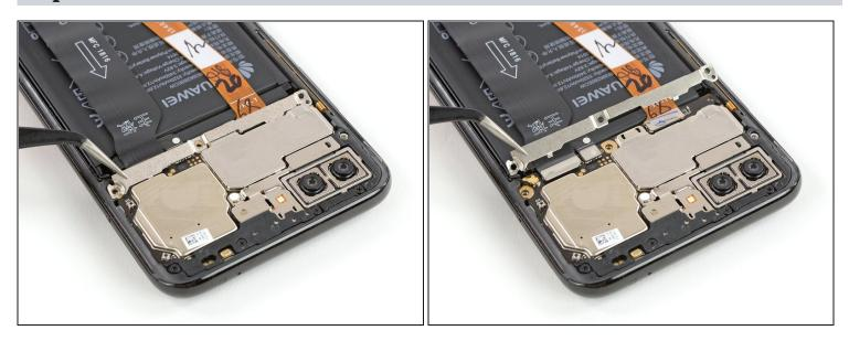
• Use a pair of <u>tweezers</u> to remove the metal shield that covers the connectors of the interconnect cable, the battery and the display flex cable.
