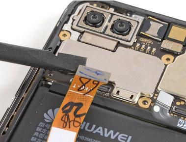
• Use a spudger to pry up and disconnect the display flex cable.
