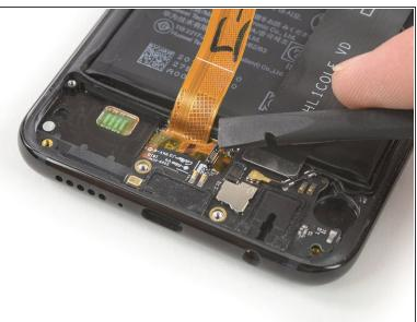
Use a spudger to pry up and disconnect the home button flex cable.
