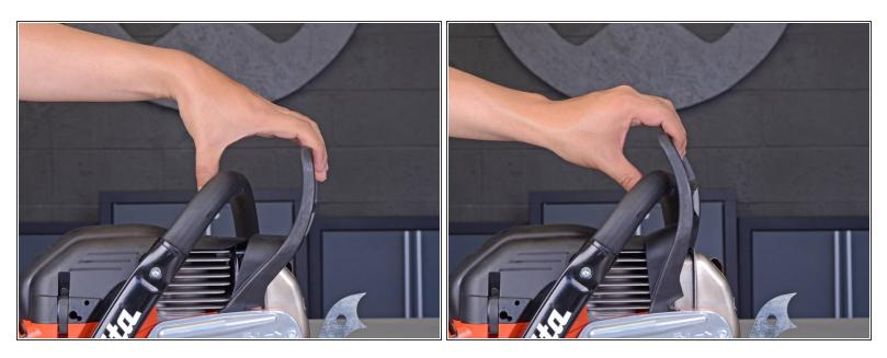
• Pull the hand guard towards the tubular handle until you hear a click to release the chain brake.
