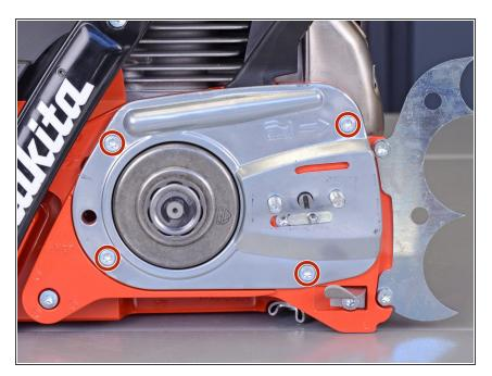
Remove the four 12 mm long T27 screws securing the chain brake cover.
