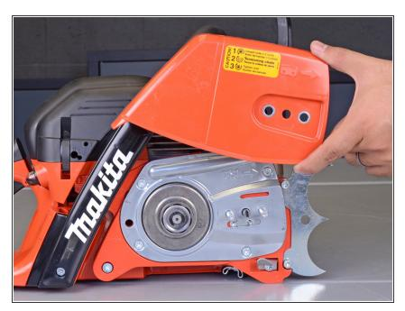
• Remove the sprocket guard plate.
