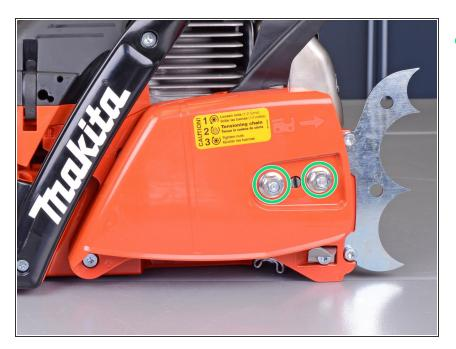
Use a 13 mm socket to remove the two nuts securing the sprocket guard plate.
