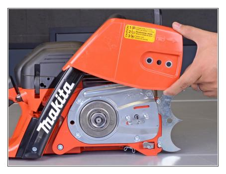
Remove the sprocket guard plate.
