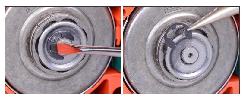
Use a small flathead screwdriver or snap ring pliers to pry and remove the stop ring from the axle.
