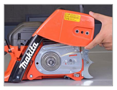
Remove the sprocket guard plate.
