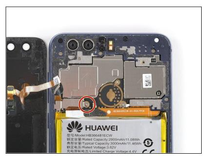
Remove the Phillips #00 screw (2.8 mm length) that secures the metal bracket on top of the fingerprint flex connector.
