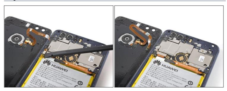
• Use a spudger to pry up and disconnect the fingerprint flex connector.
