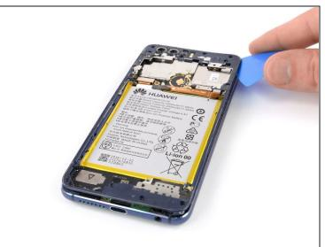
• Repeat the procedure on the right edge of the phone to cut the adhesive underneath the midframe bezel.
