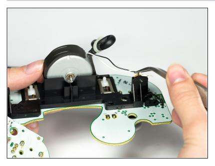
Using tweezers, unhook the wires from the small black bracket keeping them attached to the circuit board.
