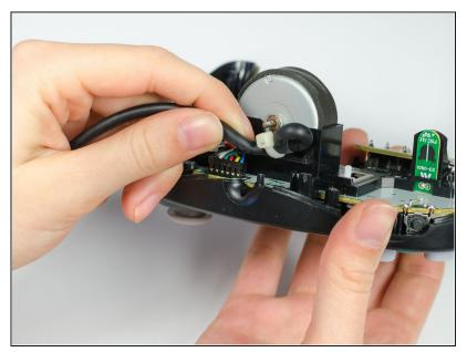
• Carefully unhook the cable that is looped around the peg.
