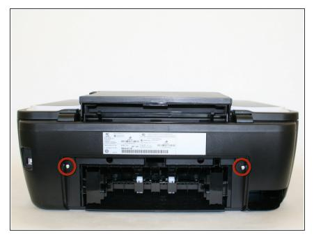
Locate the two screw holes that connect the two cylindrical extensions from the top portion of the scanner unit to the printer.
