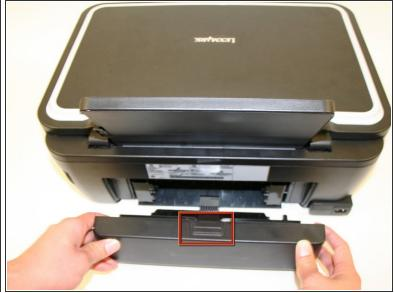
• Remove the duplex unit from the back of the printer with the duplex unit facing up.
