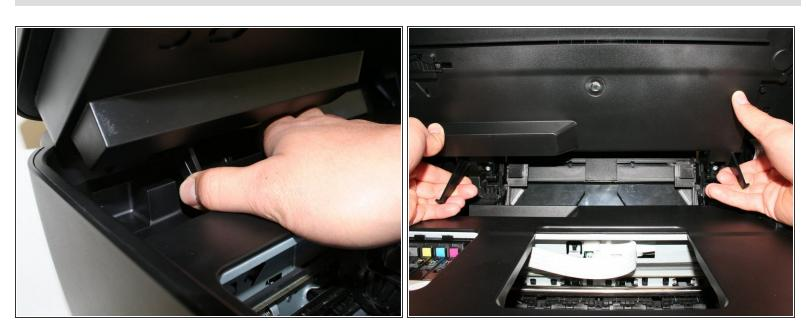
Firmly press the hinges inward toward the middle of the printer on both sides at the same time.
