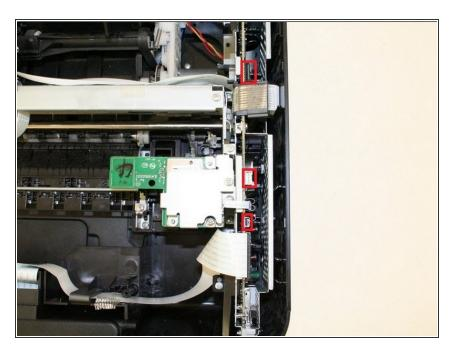
Locate the three ports for the cables from the scanner unit and make sure they are unplugged.
