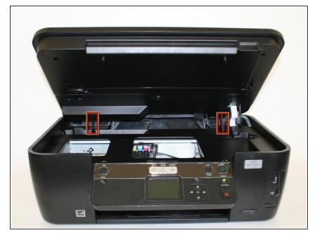
Raise and close the scanner unit to observe that the hinges lock in place when lifted.
