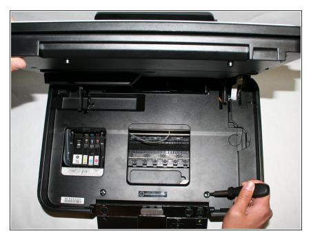
Remove the three size#6 (5-mm head) Phillips 1-mm screws connecting the scanner unit to the printer.
