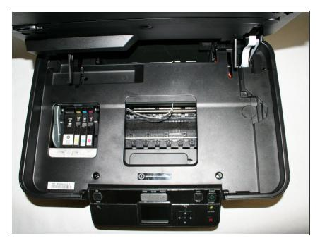
Locate the three screws connecting the plastic tray to the printer.
