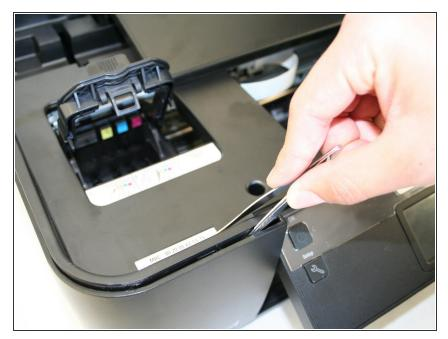
Remove the plastic cover by unlocking the plastic hinges at the inside edges of the printer. Use a plastic opening tool or a tweezer to slowly move in between the crease around the printer to unlock it.
