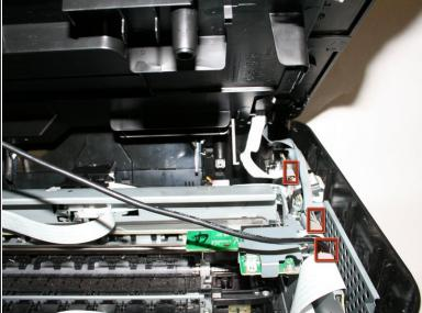
Slowly raise, but do not remove the plastic cover with the scanner unit so that it exposes the three cables connecting the scanner unit to the printer.
