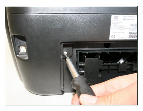
Unscrew the two size#6 (5-mm head) Phillips 1-mm screws connecting the scanner unit to the printer.
