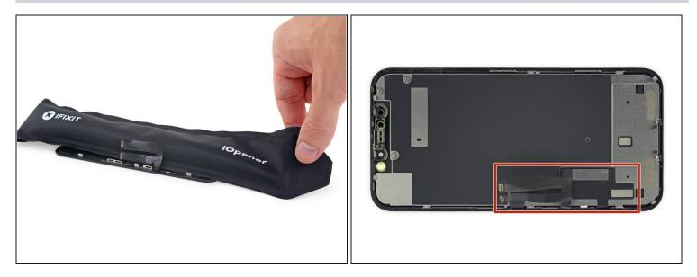
• Apply a little heat from an iOpener (or hair dryer / heat gun) to the back of the display, in order to soften the adhesive securing the display cables to the LCD shield.
