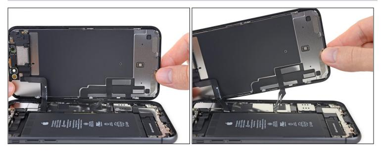
• To access the screws in the following step, tilt the display by slightly lifting its lower edge.
