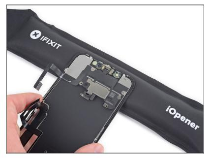
• Use a hairdryer or heat gun or prepare an iOpener and apply it to the top front of the display for 1-2 minutes, in order to soften the adhesive securing the sensors.
