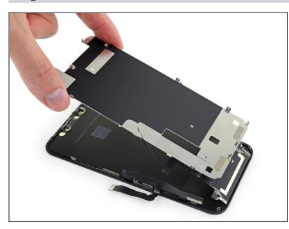
• Remove the LCD shield.
