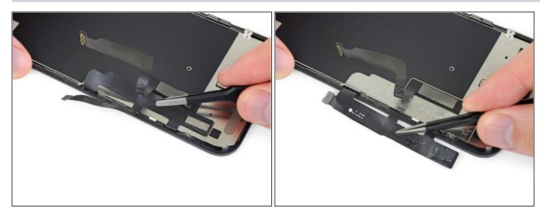
• Peel the entire digitizer cable away from the LCD shield, and fold it aside.
