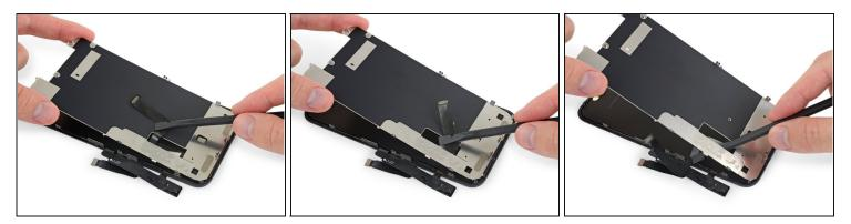
• Raise the top edge of the LCD shield a bit higher, and feed the rest of the display cable through the cutout in the shield.
