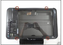
Remove the four 9mm T10 Torx screws on the top.
