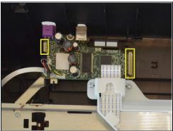
Remove the two cables by gripping each one close to their connection ports on the motherboard and gently disconnecting them.
