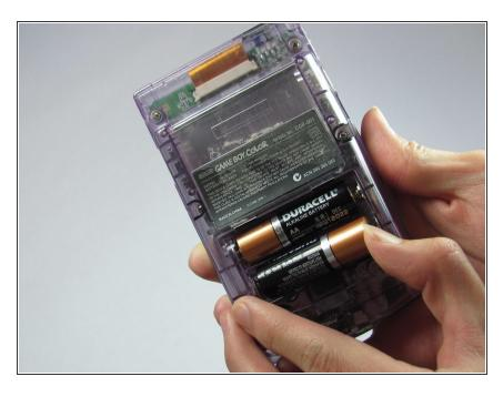
Remove the batteries from the battery compartment.
