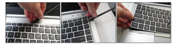
• Using a spudger, work around the edge of the keyboard and pry it up from the device.
