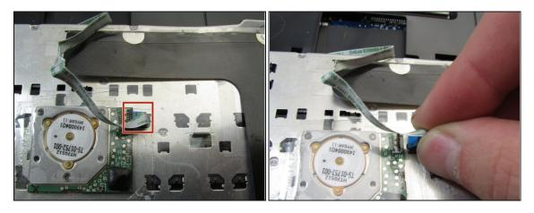
Using the spudger again, disconnect the thin ribbon strip on the back of the keyboard.
