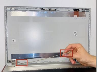
Once all the other steps have been completed you should have a disconnected LED screen, and bezel. The connector tab should remain adhered to the motherboard.
