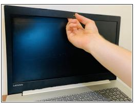
Start from the left side of the bezel (plastic covering) by gently removing inner edge of the plastic.
