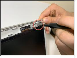
Remove the four 7mm JIS #00 screws from each corner while holding the screen in place.
