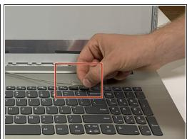
Place the LED screen on the keyboard and use your fingers or the iFixit opening tool to open the bracket securing the video connector. Then, disconnect the video cable.
