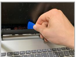
Turn the laptop sideways and insert the plastic pick between the bezel (plastic covering) and the laptop cover. Use the plastic pick to separate the bezel from the top cover.
