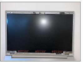
Remove the bezel (plastic covering) from the laptop completely and set aside.
