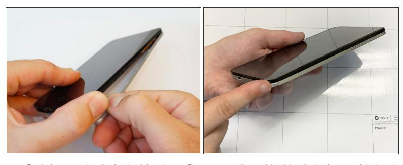
Begin by removing the back of the phone. Press your nail or a thin object in the bottom right-hand corner of the phone and gently press to release the back of the phone from the front.
