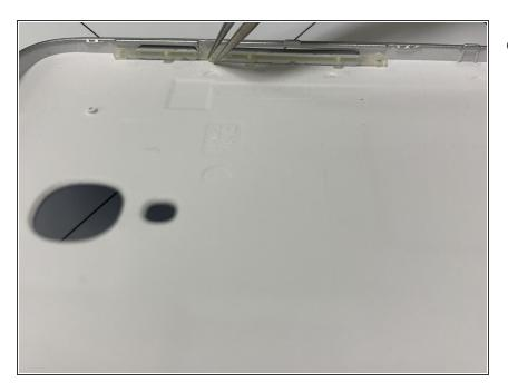
Remove the middle insert of the elastic on the Power/Volume button rocker with tweezers.
