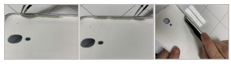
Remove the 3 elastic bands holding the rocker in place with tweezers.
