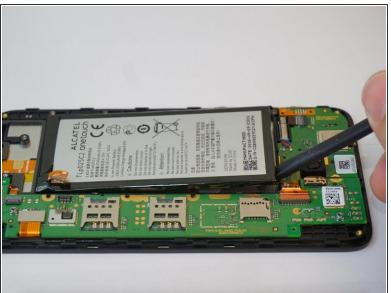
Disconnect the battery from the motherboard and remove it.
