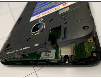
Once the screws have been taken out, remove the mid-frame protecting the phone's electronics by using a fingernail or tool to pry it off.
