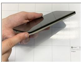
Begin by removing the back of the phone. Press your nail or a thin object in the bottom right-hand corner of the phone and gently press to release the back of the phone from the front.
