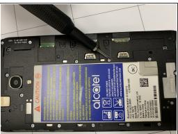
Remove seventeen 1.2 mm screws from the phone's mid-frame using the Phillips #000 screwdriver.
