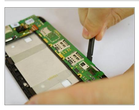
Use the flat end of the spudger to pry off the motherboard.
