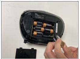
Remove the batteries located under the radio by sliding open the removable panel.
