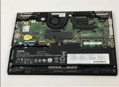
Gently remove the cover by placing your fingers around the edges.
