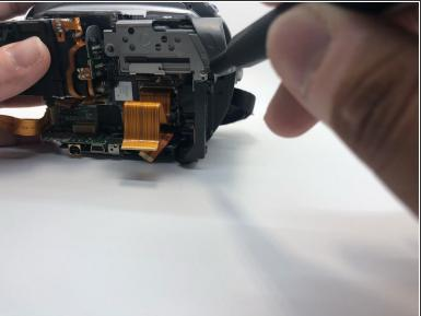
Remove the three 5mm screws on the left side of the viewfinder with your Phillips #0 screwdriver.
