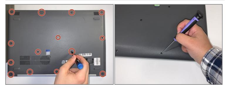
• Remove fourteen 7mm Phillips #00 screws from the back panel.
