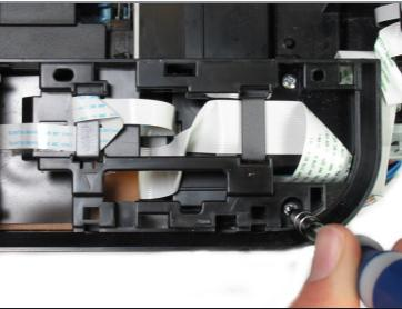
• Remove the two 7.8 mm screws using a Phillips #1 screwdriver.
