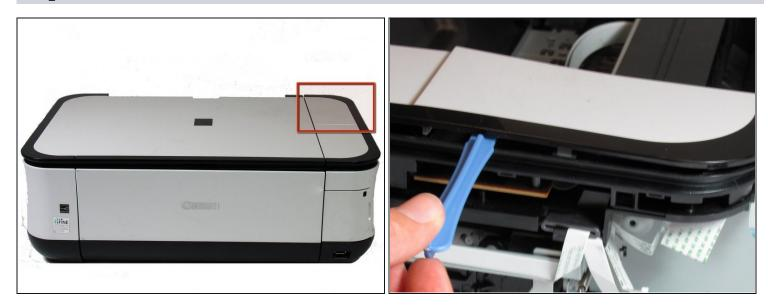
• Using the plastic opening tool, gently pry around the cover behind the LCD screen to remove it from its fixture.
