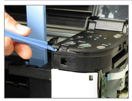
Using the plastic opening tool, gently pry under the button cover to remove it from its fixture.
