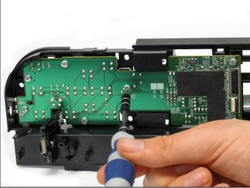
• Remove the seven 8.7 mm screws using the Phillips #1 screwdriver.
