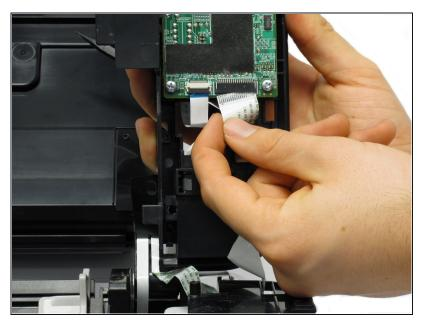
Remove the ribbon cable connected to the backside of the plastic button assembly.
