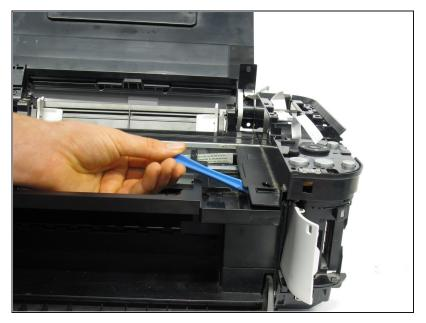
Use the plastic opening tool to pry off the plastic button assembly.
