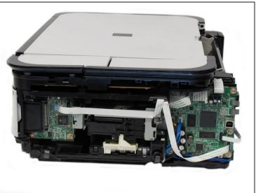
• Use the plastic opening tool to loosen the side panel from the bottom of the printer.
