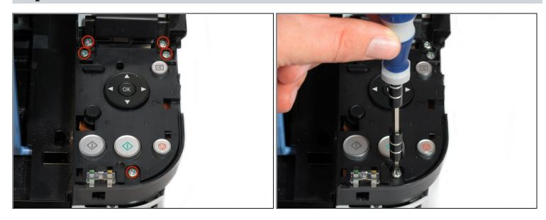
• Remove the five 7.7 mm screws using a Phillips #1 screwdriver.
