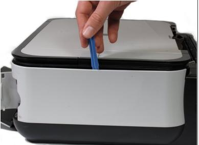
Pry open the side cover with the plastic opening tool.
