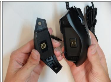
Remove the interchangeable side plate.
