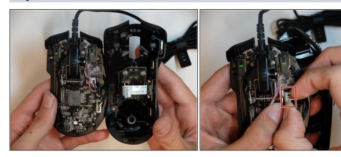
• Remove the top housing LED 3-Pin connector that is near the main board.
