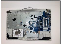
• Gently lift and remove the heat sink and set it aside.
