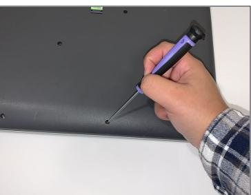
• Remove fourteen 7mm Phillips #00 screws from the back panel.
