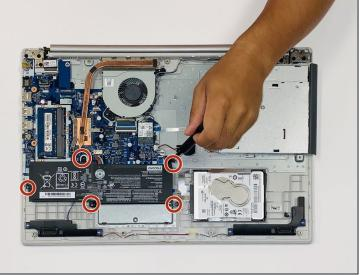
• Remove five 7mm Phillips #0 screws from the battery holder.
