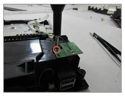
After gaining access to the boards unscrew the 3mm screws holding the Bluetooth and Wi-Fi boards in place using the Philips #0 screwdriver.
