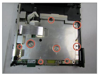
Remove the eight 7mm screws using the Phillips #0 screwdriver.
