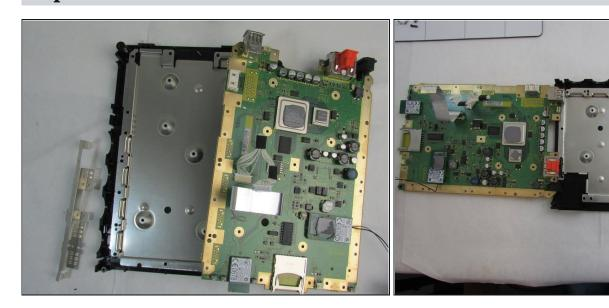
• Once the heatsink is removed, cautiously pull the motherboard out from the left side of the console case and remove it from the device.
