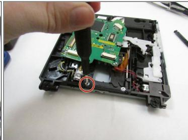
Remove the screw using a Phillips screwdriver.
