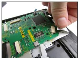
• Pinch the two cables with your thumb and index finger and pull each cable straight out from the plug-in port.
