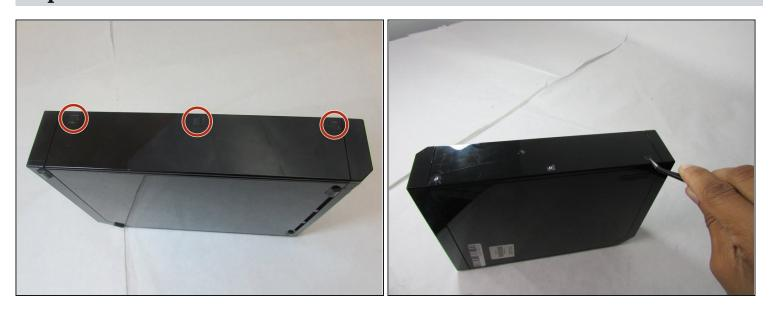
• Use <u>tweezers</u> to remove the three black square stickers on the top of the console by prying under and gently pulling up to expose three screws.
