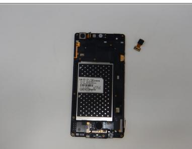
Using the nylon tipped reverse tweezers, remove the front facing camera.
