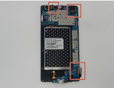
Using the plastic opening tool, carefully slide the edge of the tool under the press fit cable connections and lift up to disconnect. Do this for all three ribbon cables.
