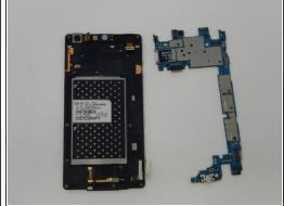
Using the iFixit opening tool, remove the motherboard from the screen by inserting the opening tool under the edge of the motherboard and lifting up.
