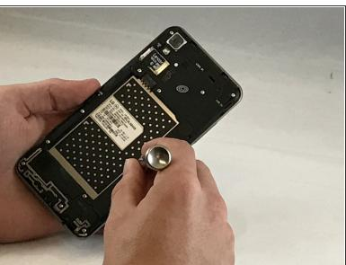
With a Phillips #000 screwdriver, remove the twelve 3mm screws.
