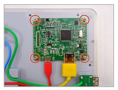
• Unscrew the four 8.5mm screws with your Phillips #1 Screwdriver.
