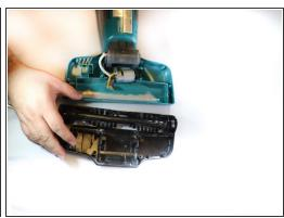
After removing all of the screws pull the vacuum's black cover up to remove it.
