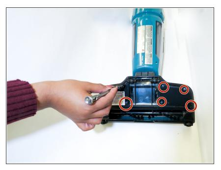
Use a Phillips #0 screwdriver to remove each screw.
