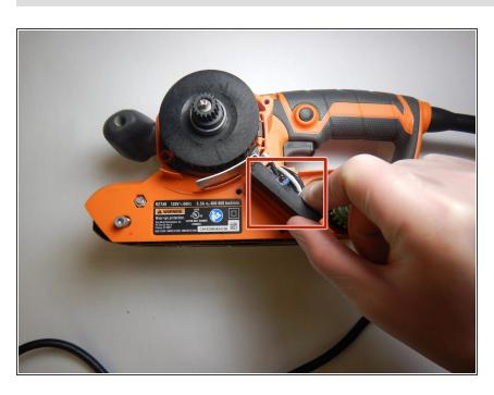
Gently pull up on the motherboard chip set, pulling it directly from the device.
